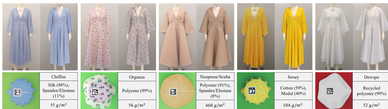
Figure 1: The line below shows Cusick drape test results and tag info for five actual fabrics. The tag information includes fabric type, fiber composition, and density. Using this data, we estimated optimal simulation parameters (stretching and bending) to replicate each fabric's drape property in a cloth simulator. For verification, we made two dresses: one with real fabric and another with the estimated parameters in a virtual environment. In the upper line, each pair consists of a real-fabric dress (left) and a virtually simulated dress (right).
